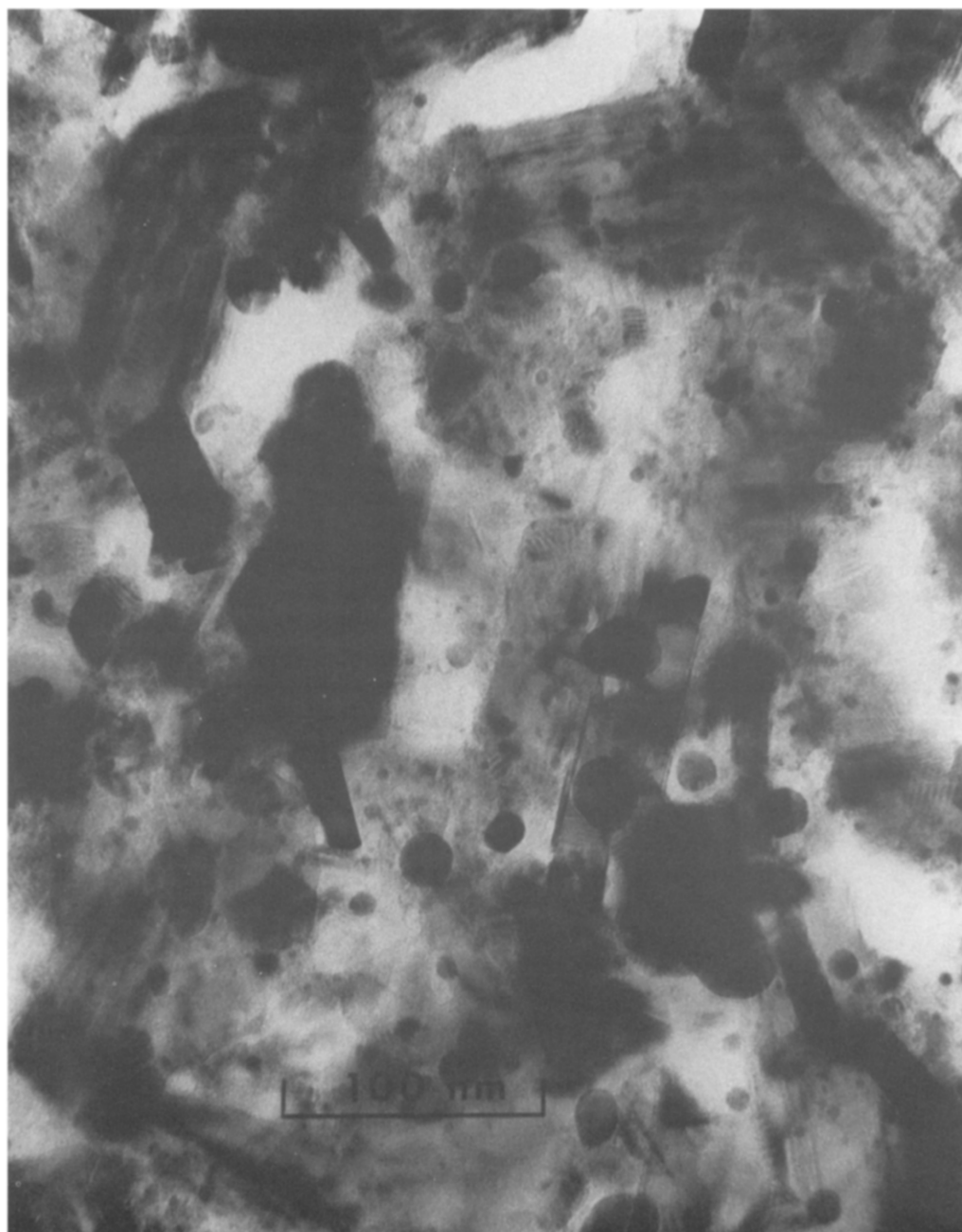
Fig. 4. Transmission electron micrograph of a Pt/titania specimen, which has been reduced at 875 K, oxidized in O_2 at 875 C, and reduced at 875 K.
